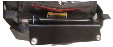
Step 2: Adjust the side clamps evenly by holding the center tube and rotating the individual clamps the same number of turns until the distance between fits inside snowmobile or ATV rear bracket.
