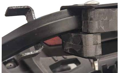
Repeat on opposite side and rotate the same plastic spacers for both sides. Tighten both wing nuts.
